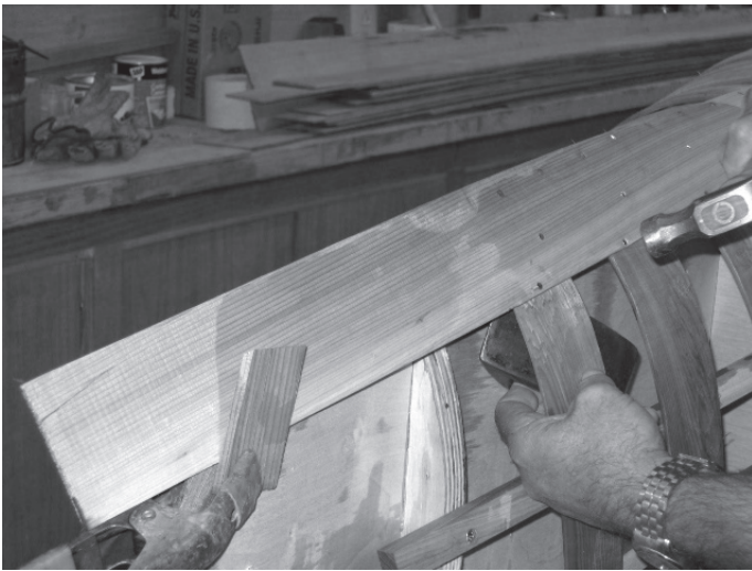
Figure 6. The garboards are wetted to make the twist at the stems.
