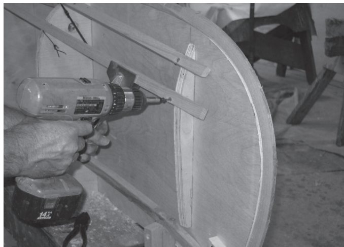
Figure 1. Screwing the ribbands to the last station.
