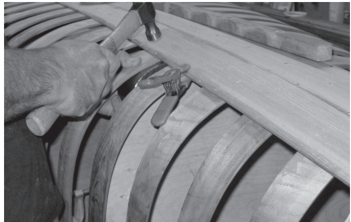
Figure 8. Using a spring clamp to hold the plank in place.
