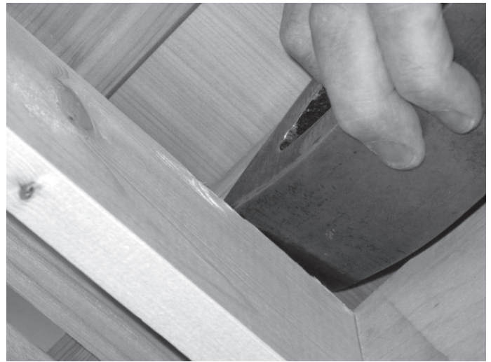
Figure 4. To clench the tacks, an iron is held under each rib.
