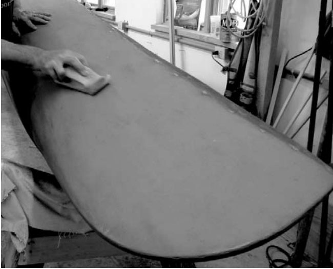
Figures 13. The last step before painting is sanding. A foam block hand sander is the ideal tool for the job.
