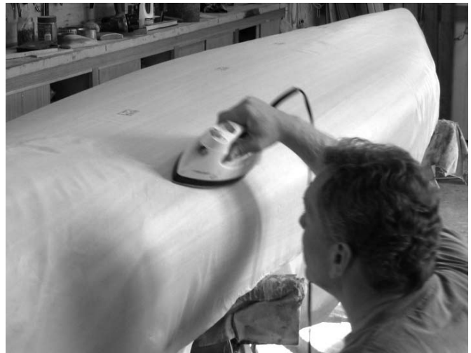
Figure 2. Using the iron to remove any wrinkles and tighten the fabric. Note the wrinkles to the left of the iron.
