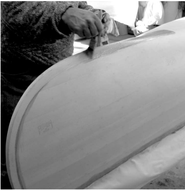
Figures 11 and 12 (above). After applying the adhesive to the bias tape at the stem (above, left), it's essential to remove the excess adhesive.
