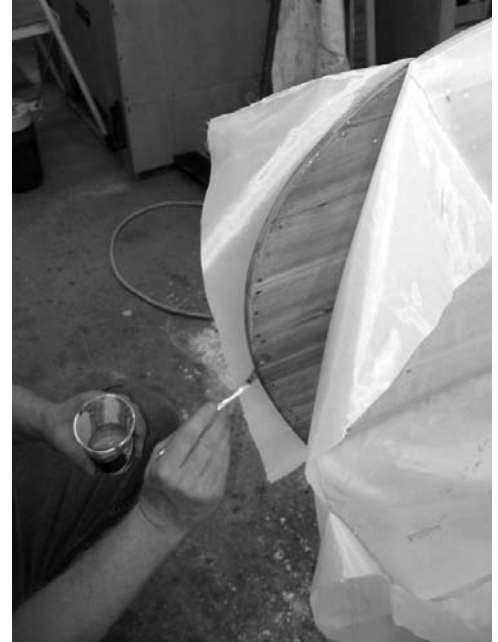
Figure 6. Once the stem is exposed the adhesive can be applied.
