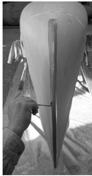
Figures 9. Applying adhesive to the Dacron bias tape.
