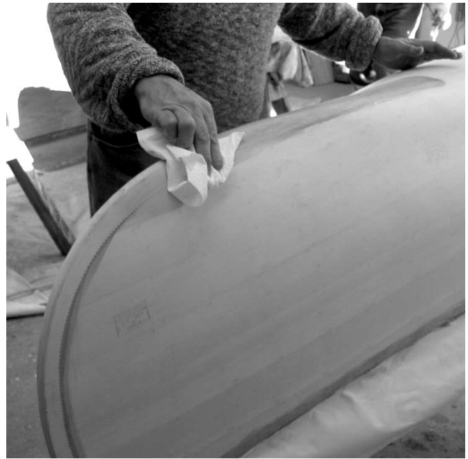
Figures 11 and 12 (above). After applying the adhesive to the bias tape at the stem (above, left), it's essential to remove the excess adhesive.
