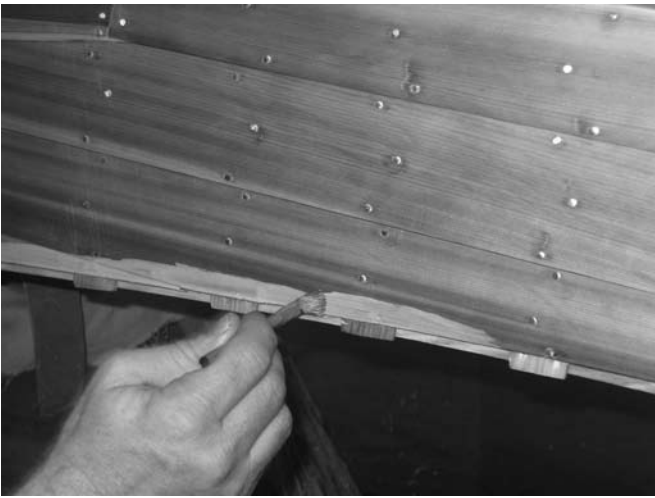
Figure 1. Applying the adhesive along the top half-inch of the planking. Two coats of adhesive will assure a good bond.
