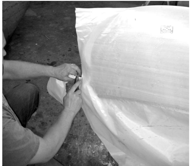
Figure 3 (below) Trimming the fabric at the stem.
