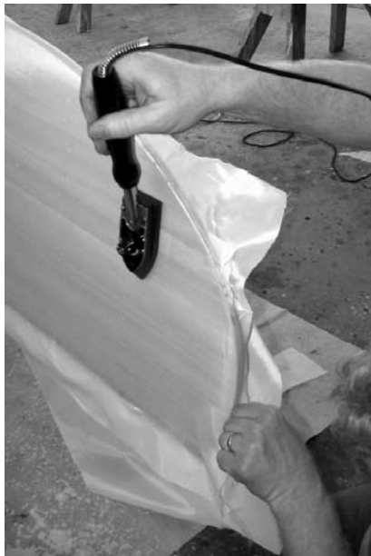
Figures 7 (above, left) and 8 (above, right). Tacking the fabric to the stem.
