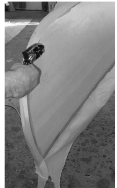
Figure 10. Using heat to activate the adhesive.
