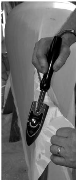
Figures 7 (above, left) and 8 (above, right). Tacking the fabric to the stem.
